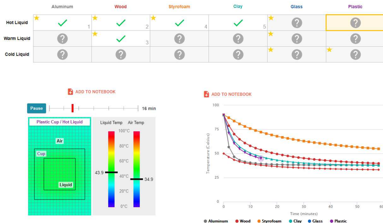
Figure 1. Screenshot of the experimentation matrix and interactive model in Thermo Challenge . Students use the matrix to plan their key trials for investigation beforehand (recorded in the matrix as “starred” tests). Students then use the matrix to run the model (completed tests are indicated with green check marks).
