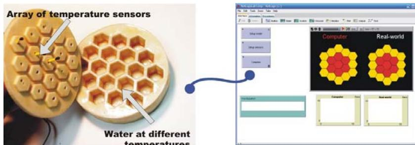
Figure 1. A 'hybrid' system for investigating heat transfer.
