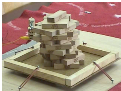
Figure 1. Sample student-designed earthquake-proof structure on earthquake simulator
