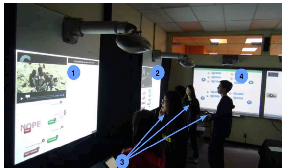
Figure 2. The smart classroom with (1) An interactive whiteboard that orients students towards a specific Hollywood scenario, aggregates scenario specific student contributions and facilitates idea negotiation; (2) A second board with a different scenario; (3) Individual tablets provide students instructions, allow them to access the knowledge base, and contribute ideas to the shared display; and (4) An ambient display showing where students are in the room, completed tasks and time left in the current task.
